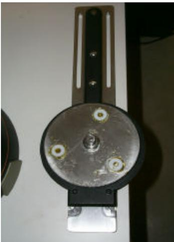
Install the Clutch disk on the OTA arm. After that install the Driven gear to the arm.
