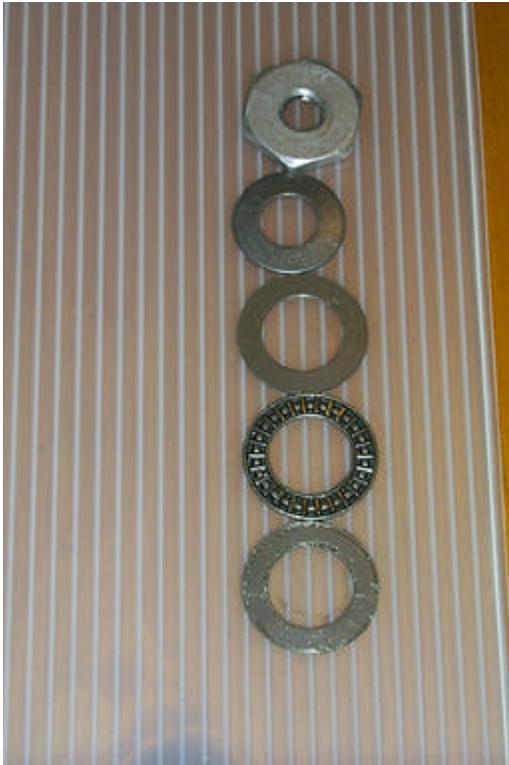
After removing the Nut you should find a conical washer and a Torrington bearing. The grease will tend to hold them into place, Remove them if you can to keep them from falling to the floor. Also try to keep them as clean as you can. (No dirt here)
