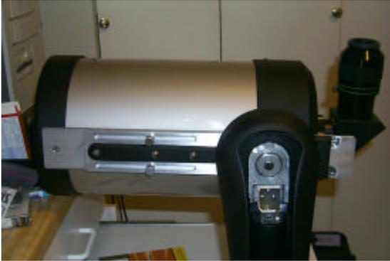
Now install the OTA to the arm. Also install your 2" diagonal and your heaviest Eye Piece. Now slide the OTA back and forth to find the balance point. On mine with a CI 2" Diagonal and a Nagler type 5 Eye Piece, the balance point is 2 1/4" forward as shown to the left.
