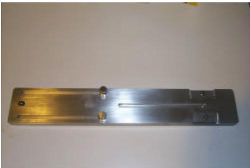
Take the new bracket, and remove the two thumbscrews.
