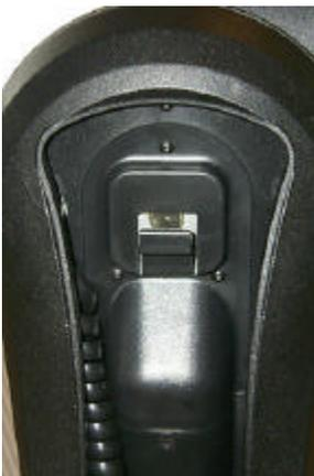
Now that the nut is adjusted, install the Dec nut cover.
