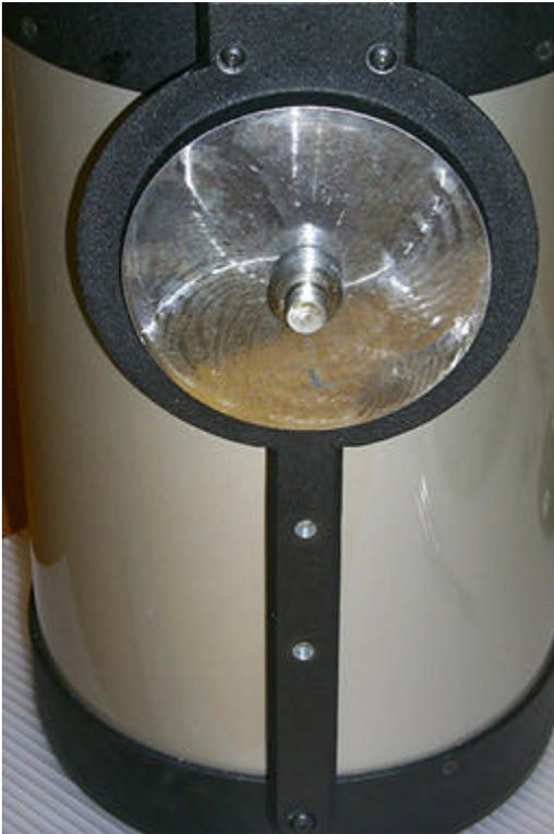
At this point if you look at the OTA you will see the OTA mount arm. It is held in place with three (3) Allen head screws. The two (2) screws at the back of the OTA are smaller than the one (1) at the front of the OTA. Remove these three (3) screws and save them for future use. **You will not be using them with the kit.**
